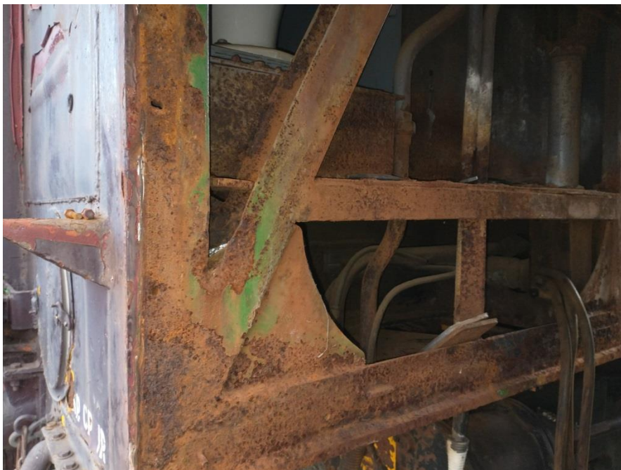
The image shows the exposed carbody framework at the back corner of GM 1. Plenty of surface rust but overall quite sound.
