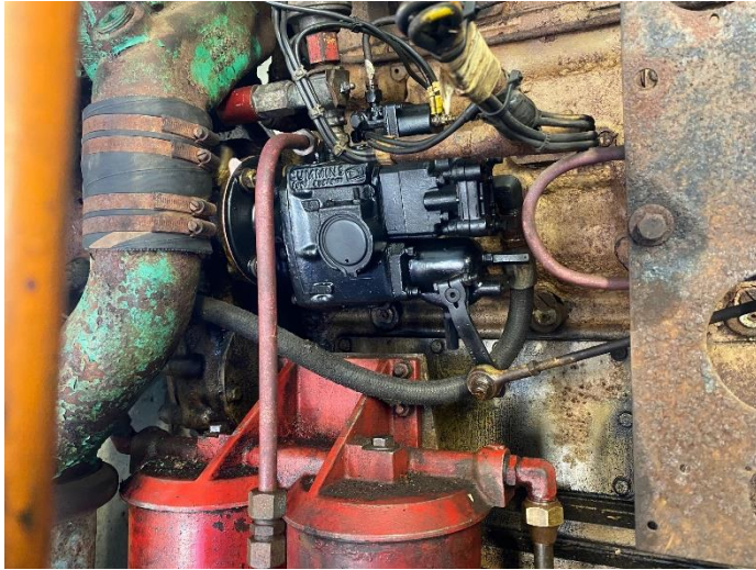
The overhauled fuel pump (painted black) is back in situ.
