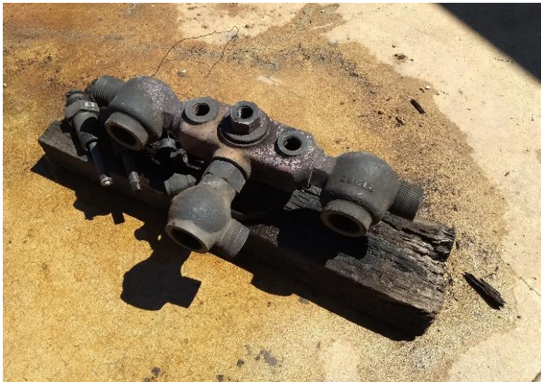
Here the crown mounting has just received a good pressure washing after going for a swim for a couple of weeks in a tub of caustic soda.
