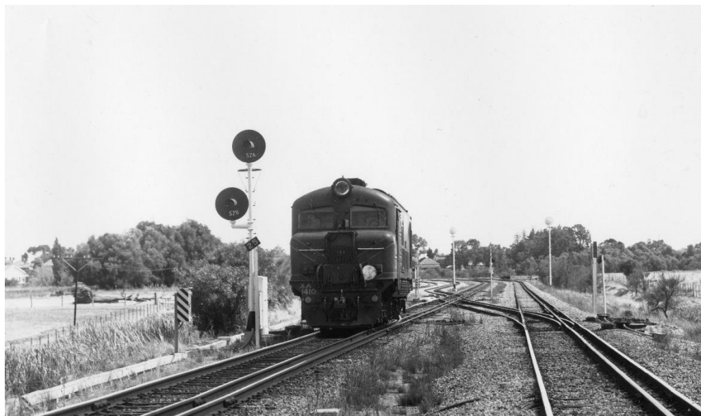
XA 1410 "TENMA" with semi- automatic colour light signals and double track cross over at Woodbridge South looking north.
