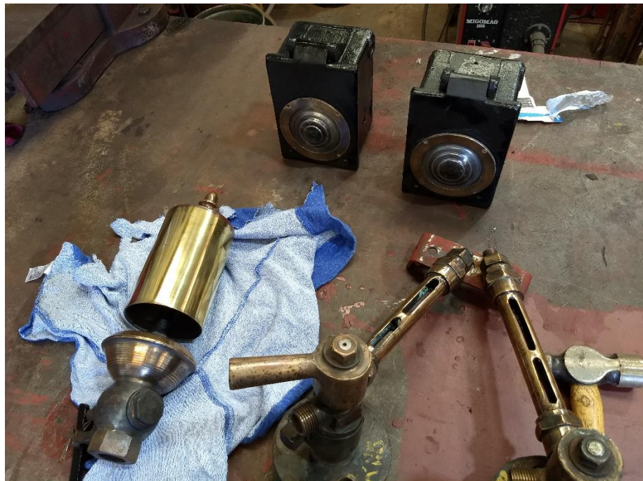
The gauge glass assemblies were all cleaned up keeping company with the whistle and marker lights.
