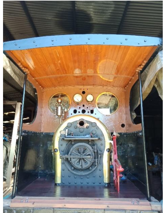
Timberwork in the restored cab of A 15 at Meredith, Victoria (Hayden Kinley)
