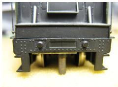
During the disassembly of the tender it became apparent that the draw bar pin on the tender had been riveted into the plastic frame with considerable force to the extent where the chassis had partially cracked and distorted resulting in a small gap between the top of the chassis and the bottom of the water tank on the right hand side – see photo above right
