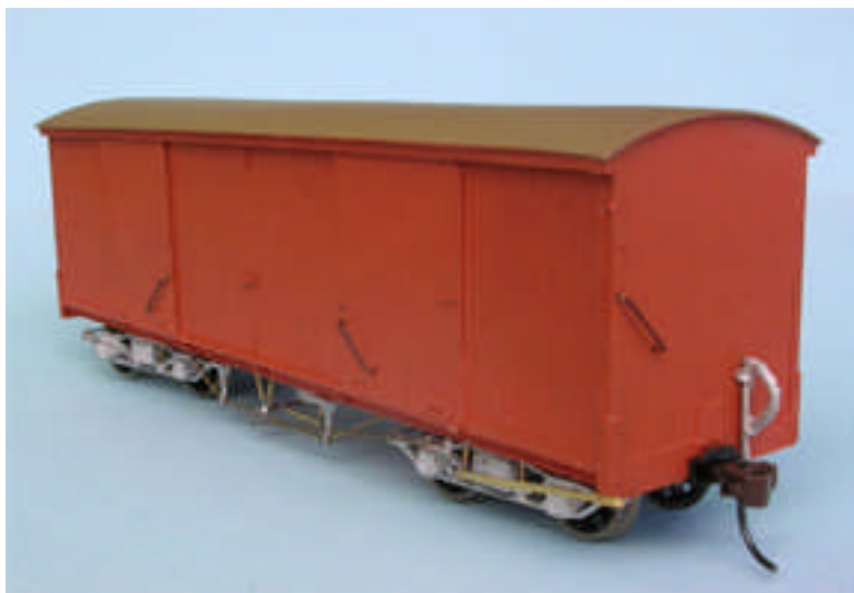
One of the new Railwest V van kits which Paul Tranter has assembled
