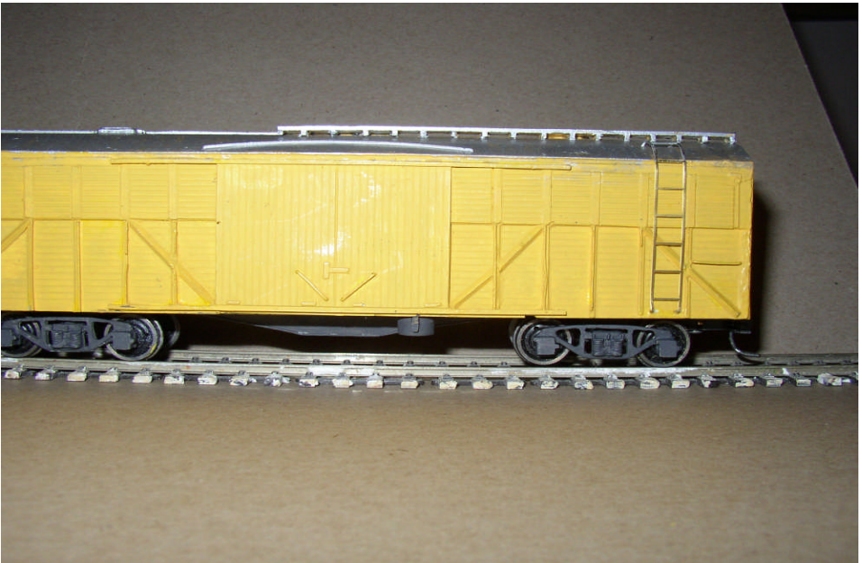
One of Greg Aitken's VFA vans modified from an X class models VF van kit with an etched brass ladder, from Model Etch.
